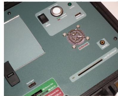
**BVM's** solution was a compact design built into a standard flight case, with a touch screen display and built in battery pack, all specially selected to be suitable for transportation on passenger airliners.
