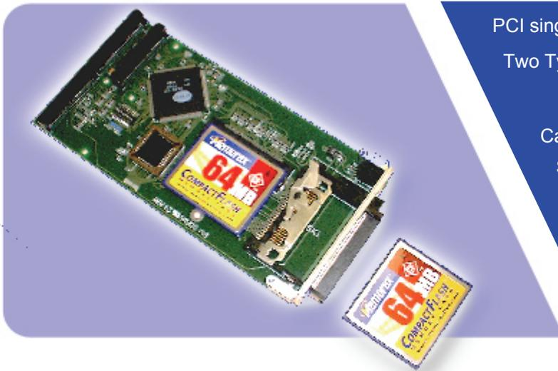
PCI single chip IDE controller (CMD PCI-648).
