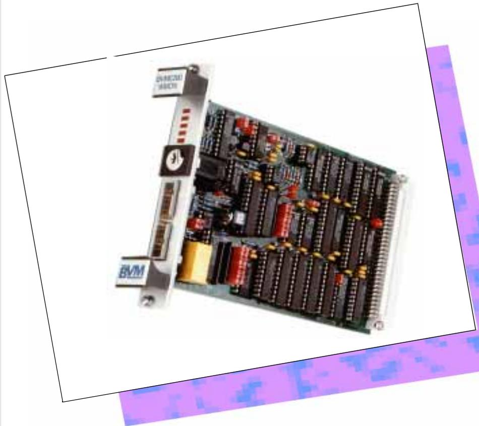
An on board rechargeable Ni-cad provides the facility of battery backup, which feeds the VMEbus +5V standby line during power down. The watchdog is user enabled in software by writing to the watchdog register. Once initialised the watchdog must be written to within a link selectable timescale of 100mS, 1S, 10S or 60S. Failure to write to the watchdog register in the set time will cause an alarm.
