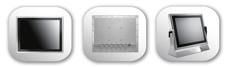
**Main System** I/O & Power & Control Keys Intel® Celeron® J1900 2.0 GHz quad-core USB processor (10W max.) COM Intel® HD Graphics LAN
