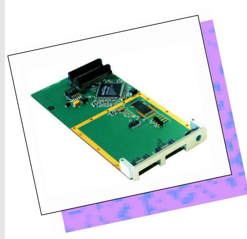
The PMCSATA features the SiL3112A Controller chip and supports both 33 and 66MHz operation achieving a maximum transfer rate of 150MBytes/sec as specified for Serial ATA generation 1.
