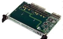
The cPC2PMC is a hot swappable CompactPCI<sup>®</sup> PMC carrier. Two PMC module sites are provided. It is possible to remove the cPC2PMC and associated PMC modules from a powered CompactPCI<sup>®</sup> system without having to power down the system first. Currently the Hot Swap features are fully supported under Windows2000 and XPEmbedded.
