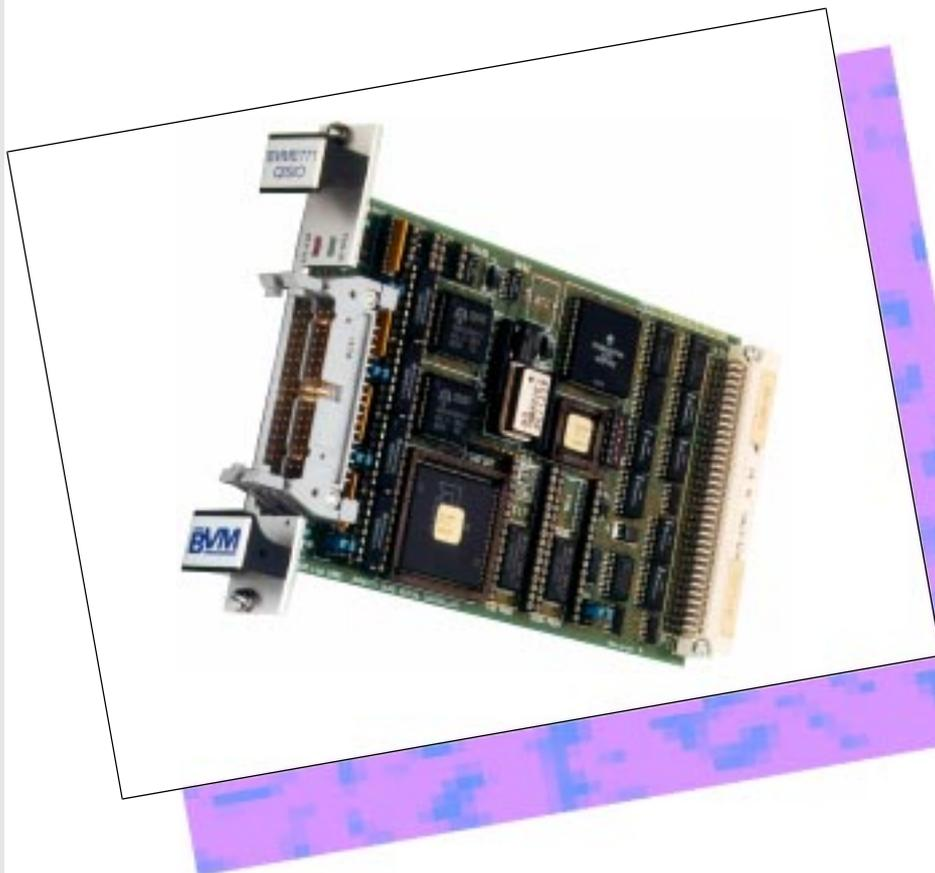
Both the BVME771 and BVME772 are based on a 68HC001 16-bit processor, a low power CMOS member of the 68000 family. Communication with the VMEbus is via a high speed dual port SRAM buffer.
