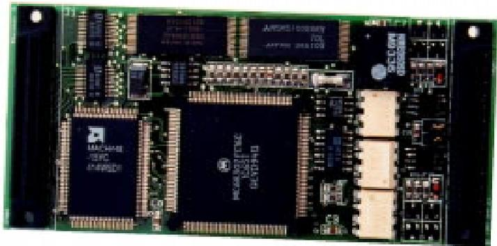
The IP302 is optimised for use as a gateway into BVM's FieldLink distributed fieldbus network but it finds many applications in other communication areas where the microcode of the 68302 offers many advantages.
